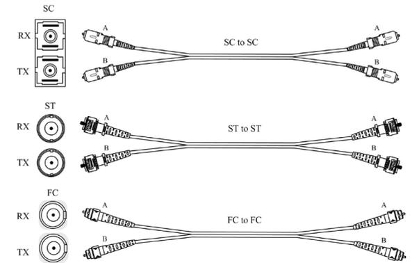
**Suppose:** If you make your own cable, we suggest labeling the two sides of the same line with the same letter (A-to-A and B-to-B, shown as below, or A1-to-A2 and B1-to-B2).
