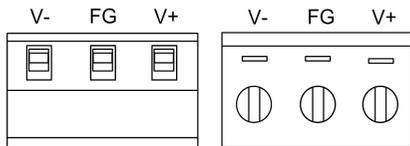
USB232/485/422 can plug and play, external power supply or USB port provide power or both of them. Power input has 3 bits terminal block (V-, FG, V+), V-, V+ is 9VDC~48VDC. The power supply support non polarity, It can work steadily if connection opposite too.
